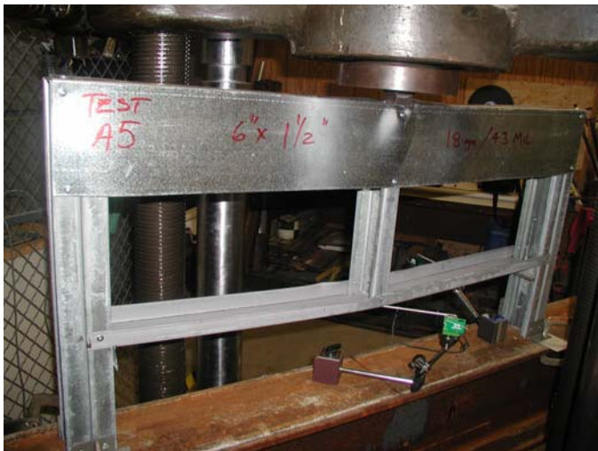
Figure 5 – Failure of Single L-Headers Tested Assemblies
